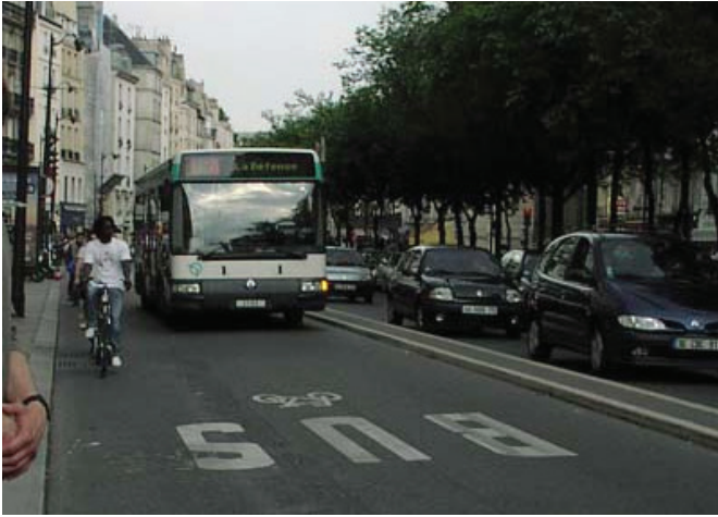
Figure 76: Cycling on shared bus lane with space for overhauling, Paris (France)
