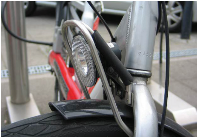
Figure 28: Robust built headlight of “DB Call a bike” Source: Hefter 2011
