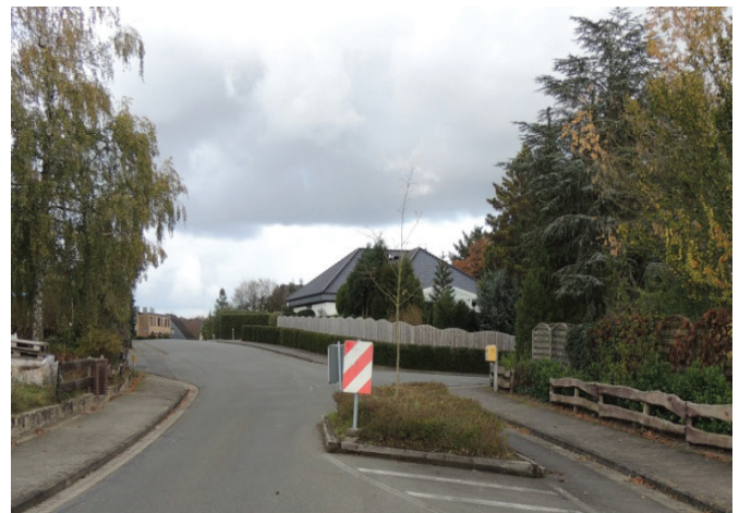
Figure 42: Horizontal deflection forcing cars to yield Source: Fricke 2012
