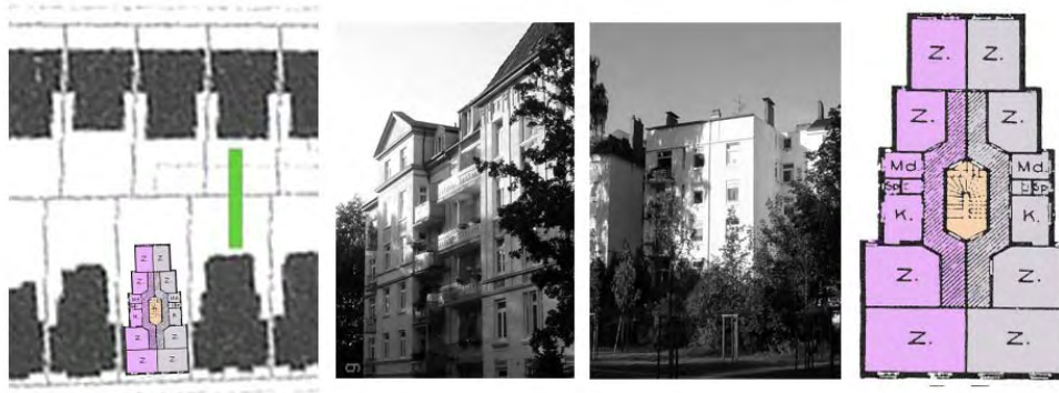
Figure 7: Example of „Schlitzbau“, minimum space of backyard shown by green bar, the ground plan shows two flats with rooms oriented only to the narrow space between the volumes, the so called”Schlitz“, using topographical maps, photos, ground floor (photo: Auraplan).
