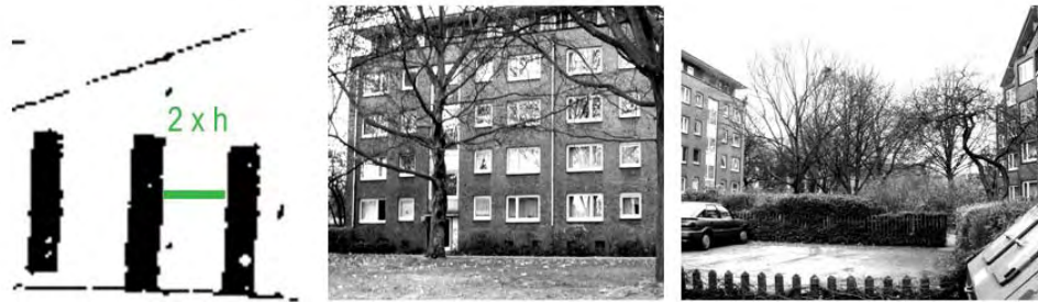
Figure 8: Minimum space between the houses as set by actual legal requirements in Germany, (Landesbauordnung-building regulations of the federal states), and shown by the green bar, is a relation of 2 times heights of the buildings. Using topographical maps (photos, ground floor, Auraplan).
