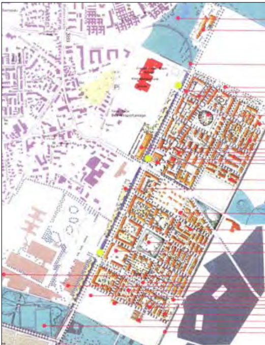
Figure 14: Entirely new quarter along the new tram line, yellow signs show tram stops. Commercial areas with working places are near the residential area, and are shown as big red forms west of tramline. Space saving building forms, there are no detached houses.
