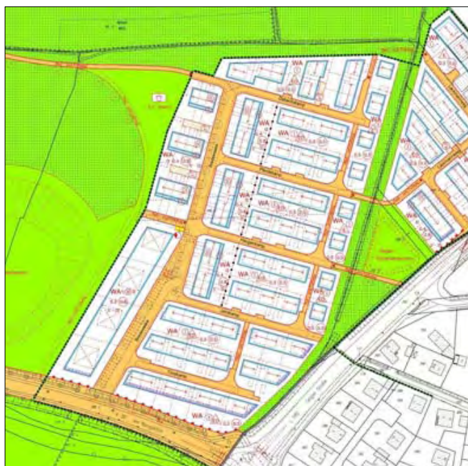
Figure 13: Example of a standard checked detailed urban plan: Building lines fix orientation mostly to the south, but not strict. Compactness is a must, but not to strict, and some detached houses are allowed.
