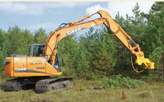
Forest guillotine used for cutting pine trees and bigger junipers
